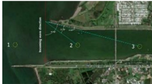
Figure 10. Inspection points of wave diffraction from north direction
